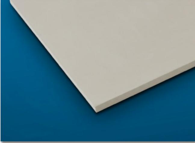
The PROMALIGHT®-1000X HD is a microporous insulation board with very good thermal and mechanical properties. The formulation is an opacified blend of filament reinforced pyrogenic silica (alumina for 1200 grade).
