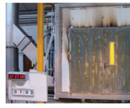
As well as controlling the exposure temperature, the test standards require that the air pressure within the test furnace is maintained at a positive level in an attempt to create a worse case scenario and force hot gases and flame through the specimen under test. Thermocouples are fixed to the unexposed face of the specimen to measure the insulation against heat provided by the construction.
