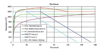
The Standard Cellulosic Time-Temperature Curve (ISO 834) This ISO-based curve is used in standards throughout the world, including BS 476, AS 1530, DIN 4102, ASTM and the new European Norm (BS EN 1363-1). It is a model of a ventilated controlled natural fire, i.e. fires in a normal building. The temperature increase after 30 minutes is 842°C.
